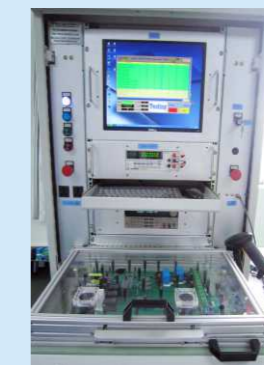
Automatic PCBA ATE test platform
