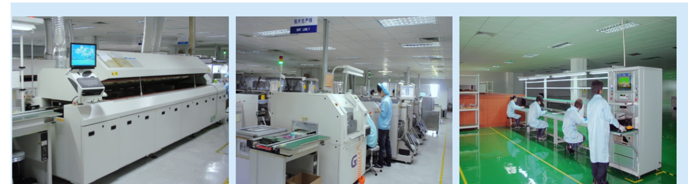
PCBA Production Line and Test
