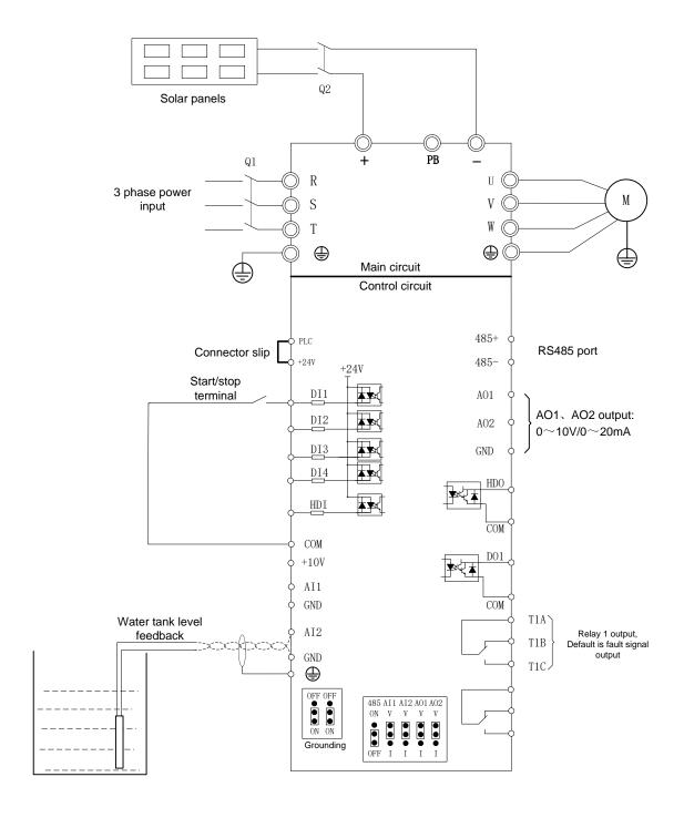
Wire Diagram of solar pump inverter
