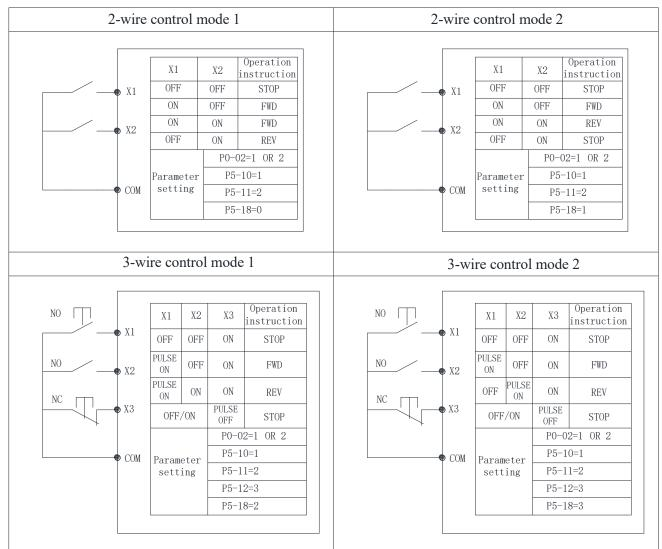
Tips: As for two-wire control mode, with the premise of the following two points, even control terminals FWD/REV remain enabled, converter will not be running any more after stop signal disappears:
