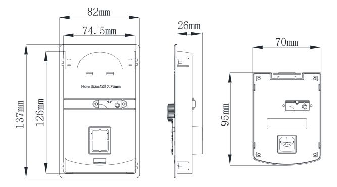
%: Keyboard base pallet hole size: width: 74.5mm; Length: 126 mm
