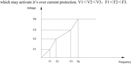
P4-07Torque upgrade $0.0 \sim 15.0\%$ Default: Depending on modelImage: This parameter can make compensation for output voltage when converter is running in a low<br/>frequency, so that the characteristics of low-frequency torque which is controlled by V/F can be
